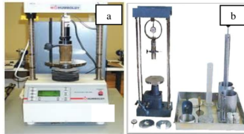
Figure 2. Test equipment a) unconfined companion strength, b) CBR test.
